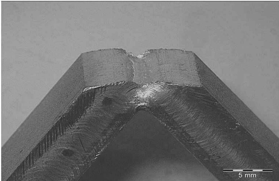
**Figure 2:** Untreated aluminium AA1200 after impact test.
