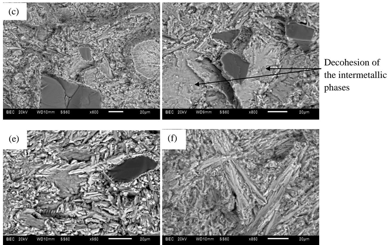
**Figure 5:** SEM fractographs of the samples laser alloyed with (a) 20wt%Ni + 30wt%Ti + 50wt%SiC, (b) 20wt%Ni + 40wt%Ti + 40wt%SiC, (c) 33.3wt%Ni + 33.3wt%Ti + 33.3wt%SiC (d) 50wt%Ni + 20wt%Ti + 30wt%SiC, (e) 60wt%Ni + 30wt%Ti + 10wt%SiC, (e) 10wt%Ni + 70wt%Ti + 20wt%SiC. (a-d) are alloys with high SiC content ( $\geq 30\text{wt}\%$ ) while (e-f) are alloys with low SiC content ( $< 30\text{wt}\%$ ).
